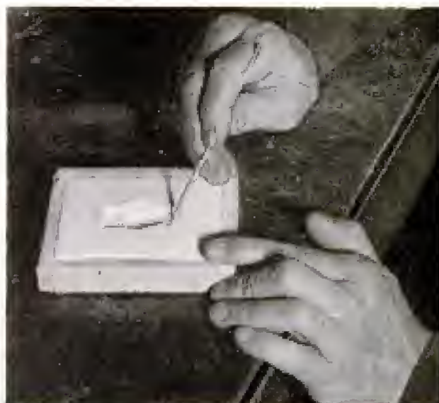
First step in making original cast is to pencil outline of figure on block of plaster. Homemade engraving tool is used to dig cavity out of block. Finished articles add humor to clothes, house plants, flower arrangements
